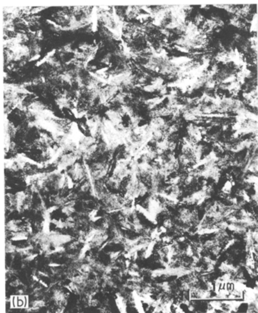
Figure 4 (a) Electron diffraction pattern from the implanted layer in a P^+ implanted specimen following annealing at 250^\circ\text{C} for 6 h showing its fine-grained polycrystalline nature. (b) Bright-field micrograph corresponding to Fig. 4a showing the morphology of the recrystallized polycrystalline layer. (c) A dark-field micrograph obtained by imaging a segment of the bright diffraction ring in Fig. 4a showing shape of the individual crystallites.
